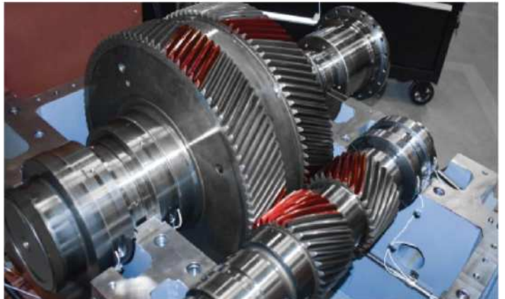
GEAR BOXES FOR UNDERGROUND CONVEYOR
