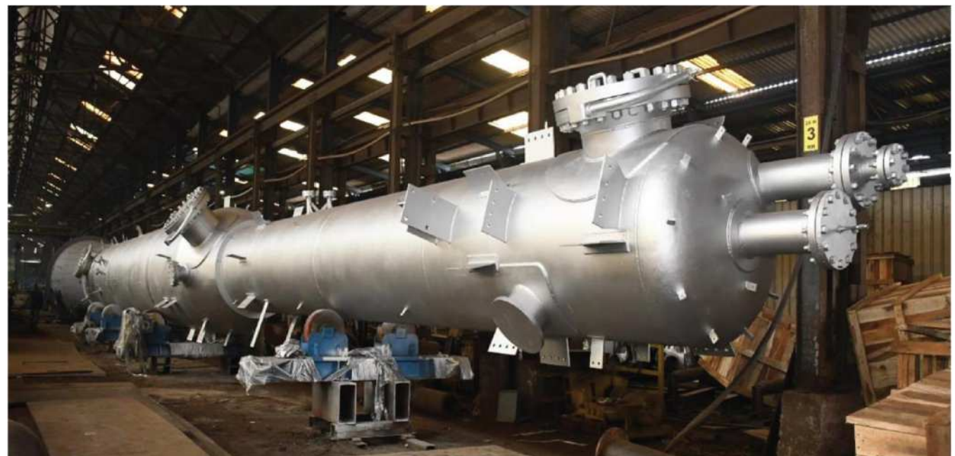
PROCESS COLUMN AT IOCL - 40M LONG
