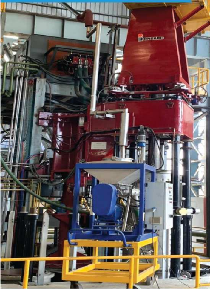
ELECTROSLAG REMELTING (ESR) FURNACE METAL & STEEL FACTORY FOR MINISTRY OF DEFENCE AT ICHHAPUR
