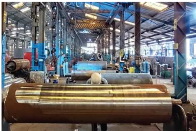
PULLEYS FOR UNDERGROUND CONVEYOR
