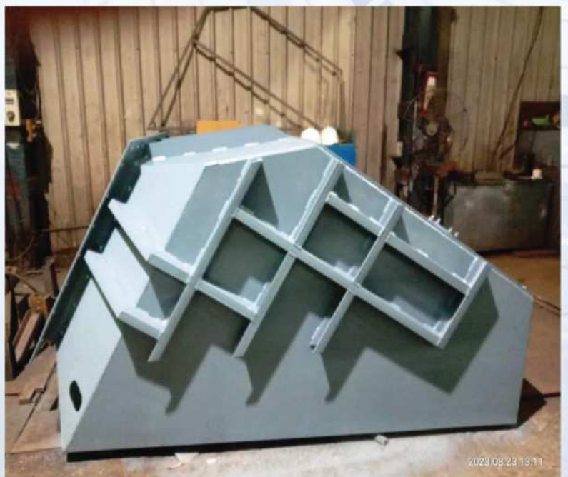
FEED GATE ENCLOSURE
